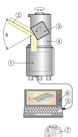
The range finder electronics (1) of the 3D scanner *RIEGL* LMS-Z360i is optimized in order to meet the requirements of high speed scanning (fast laser repetition rate, fast signal processing, and high speed data interface).
